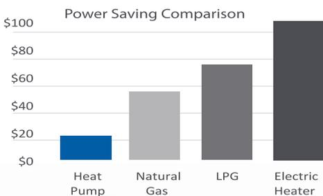
This means a Powersmart heat pump will use around 75% less energy than a standard electric spa heater and 55% less energy than natural gas. The massive saving in electricity allows you to cost effectively keep your spa or swim spa at temperature and ready to use all year round, or cost effectively extend the swimming season of your swimming pool.
